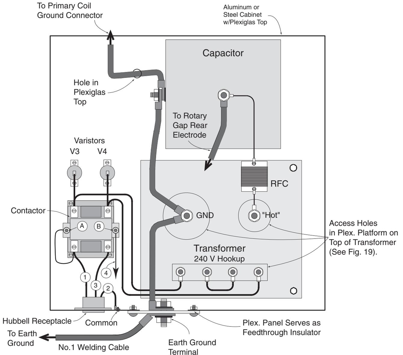
**Fig. 20 - Oscillator Top View**
