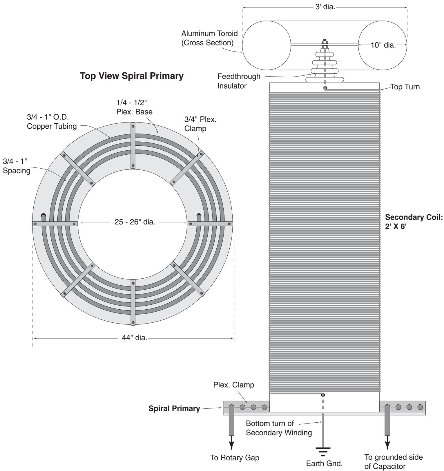
**Fig. 45 - Straight Solenoid Secondary Coil and Flat Spiral Primary**
