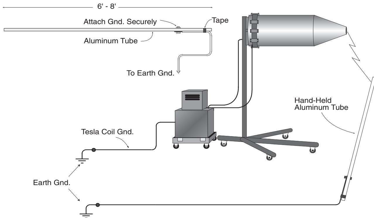
**Fig. 37 - Hand-held Discharge Arrangement**
