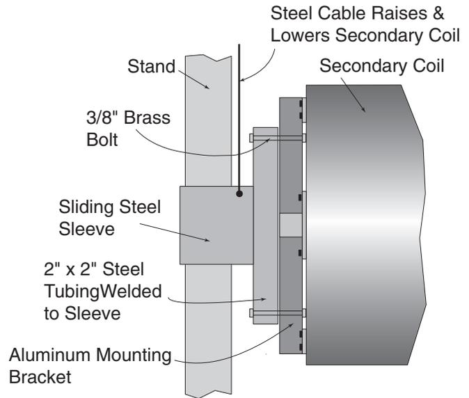
**D. Side View: Secondary Coil Attached to Vermette**
