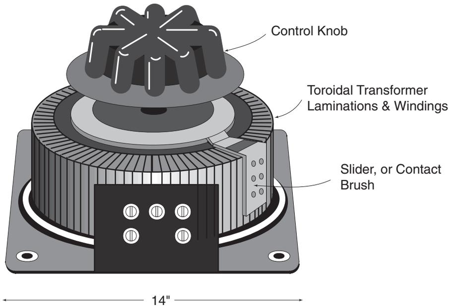
A. Typical variable transformer. Some units allow control knob to attach to either side, permitting flush mounting on a vertical or horizontal surface.
