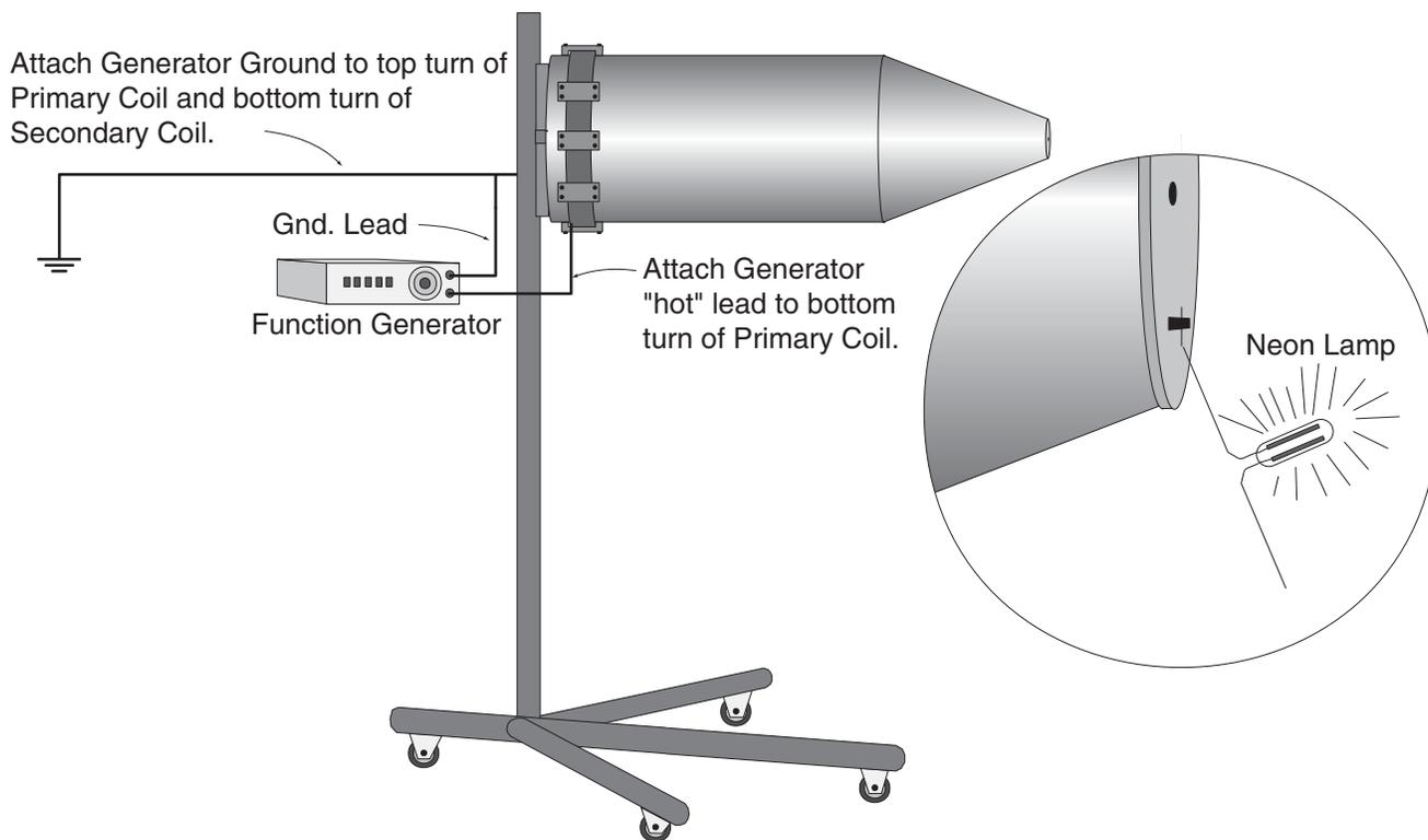
**Fig. 33 - Determining Resonant Frequency with a Function Generator**
