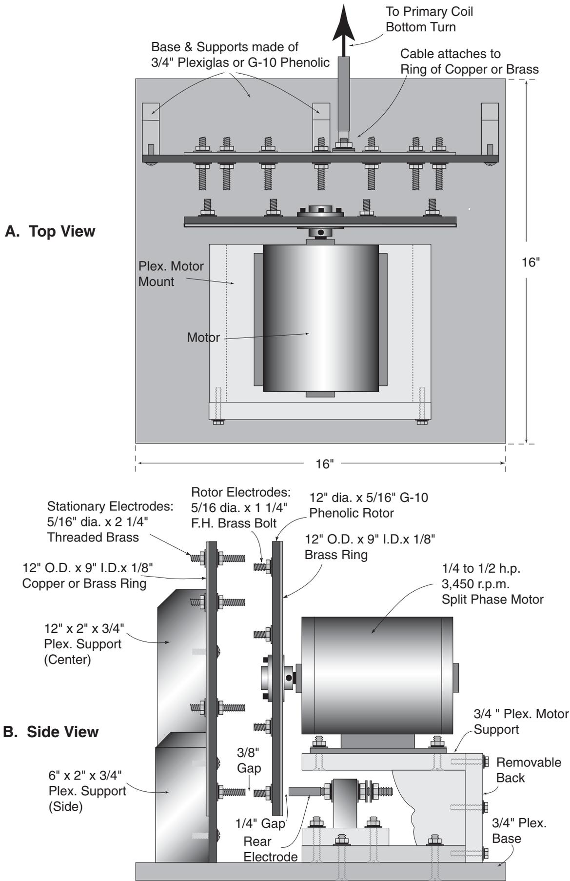
**Fig. 23 - Rotary Spark Gap**
