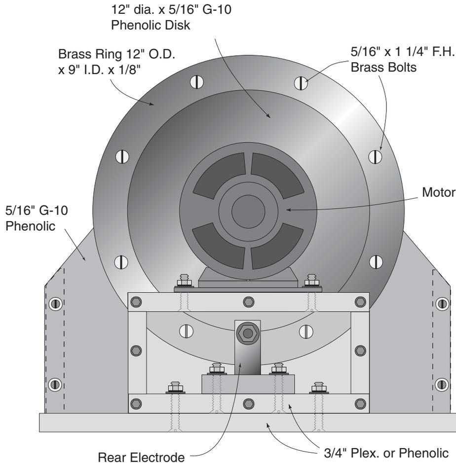
**Fig. 24 - Rear View of Rotary Spark Gap**
