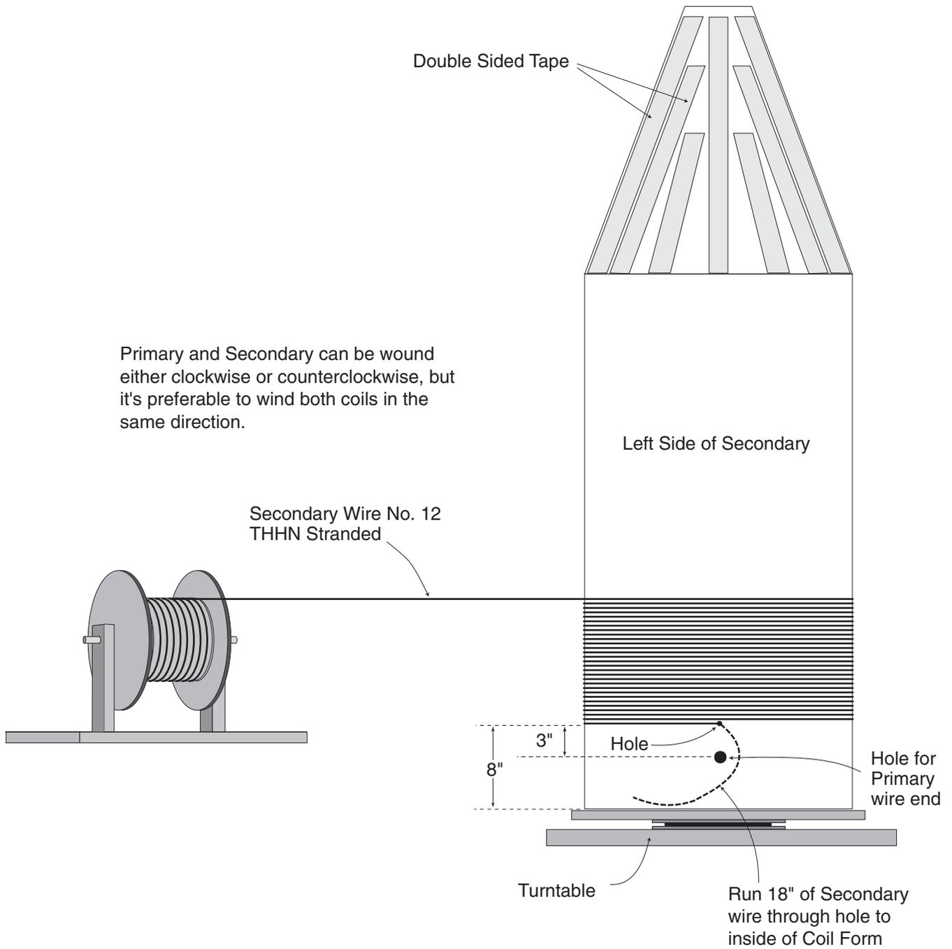
**Fig. 11 - Winding the Secondary Coil**
