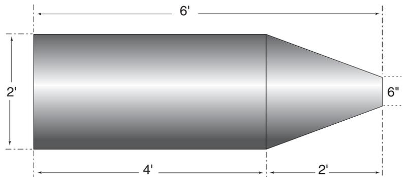
Fig. 7 - Secondary Coil
