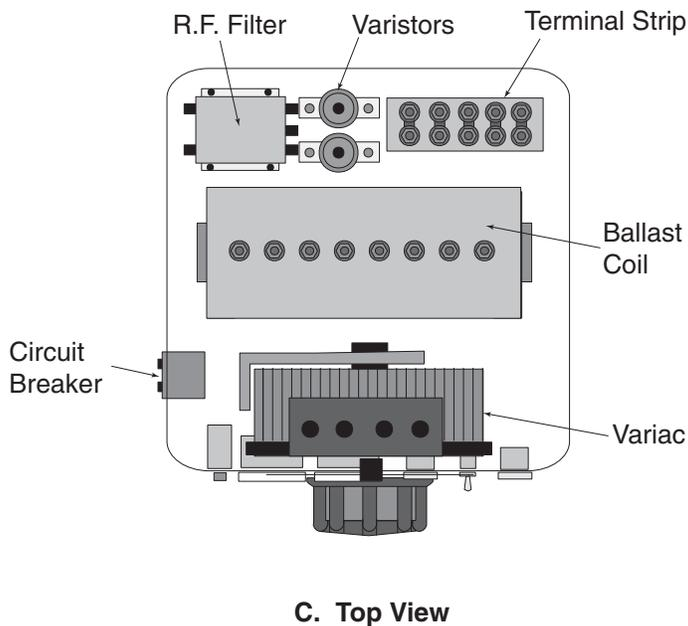
**Fig. 21 - Control Box Layout**
