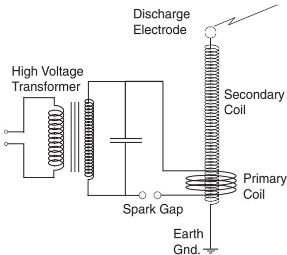
**Fig. 5 - "Classic" spark-gap Tesla Coil circuit with Secondary Coil grounded at one end and primary circuit tuned to 1/4 the frequency of the Secondary Coil.**
