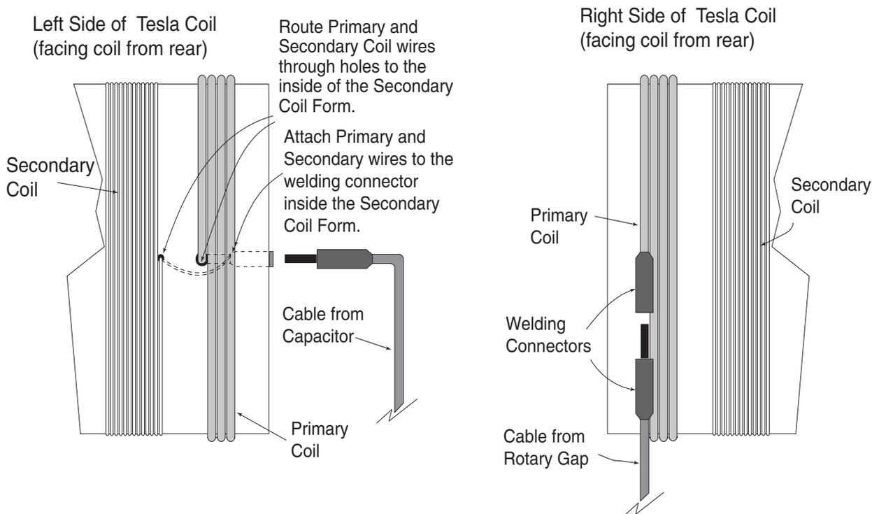
**Fig. 13 - Primary & Secondary Connections**
