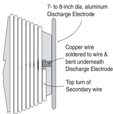
**Fig. 12 - Secondary Winding Termination**
