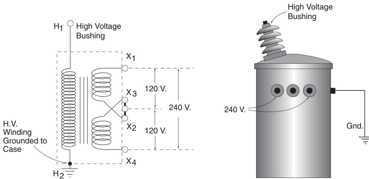
**Fig. 28 - Typical Distribution Transformer. These transformers vary in configuration and construction. Make certain that the transformer has adequate ratings and that the connections are correct.**
