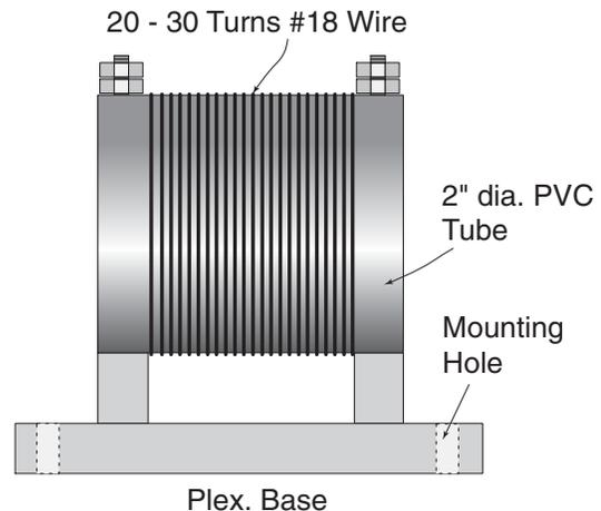
**Fig. 44 - Radio Frequency Choke reduces RF kickback from Tank Circuit**
