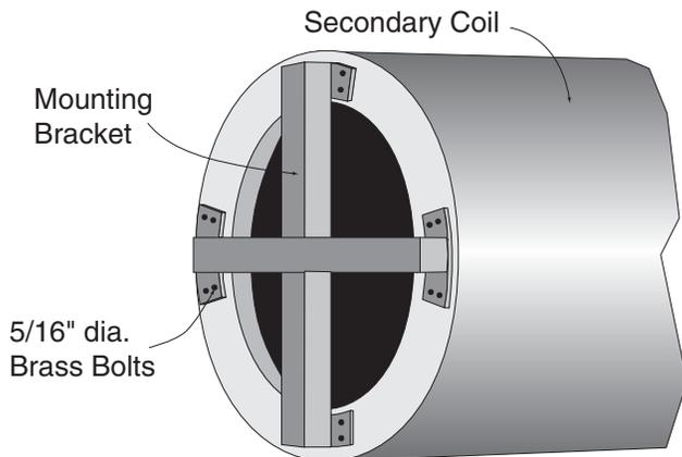
**E. Mounting Bracket Bolted to Rear of Secondary Coil**
