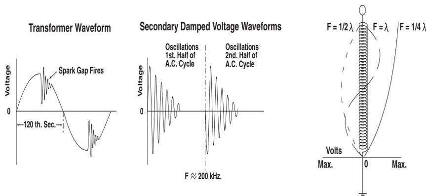
**Fig. 6 - Waveforms and Secondary voltage gradients for different wavelengths.**
