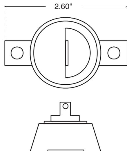
**Fig. 42 - GE Metal Oxide Varistor type V150PA20C. This model can dissipate up to 70 Joules for a millisecond. Larger models are available.**
