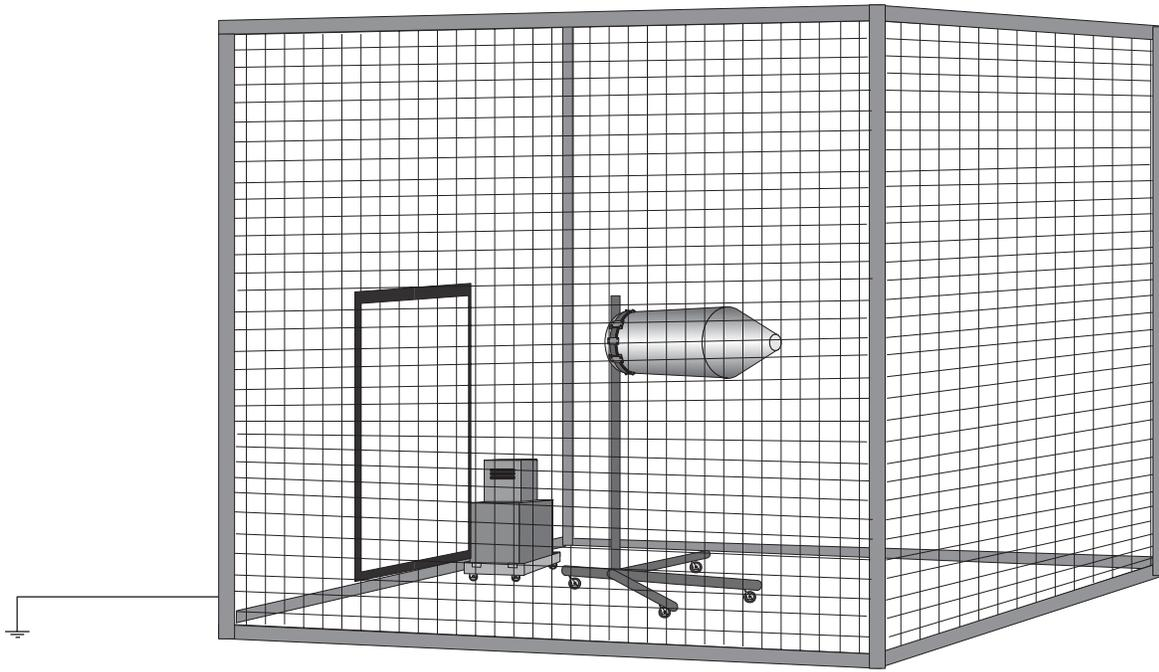
**Fig. 41 - Tesla Coil inside Faraday Cage**
