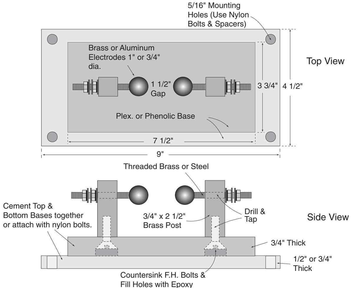
**Fig. 43 - Safety Gap protects Capacitor and Transformer against potentially damaging transient voltages generated in the Oscillator circuit.**
