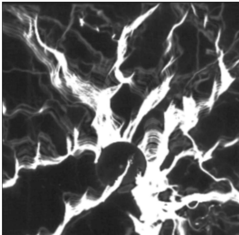
**Fig. 35 - Close up of discharge shows individual parallel sparks that comprise the larger channels. The author has no explanation of why the channels tend to form spiral paths.**
