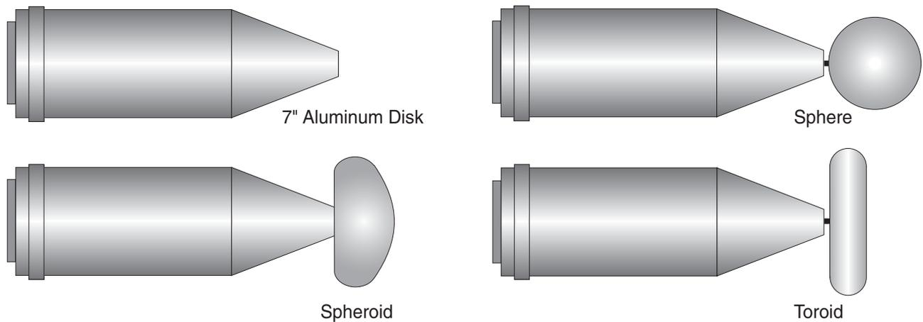
**Figure 29 - Discharge Electrode Styles**
