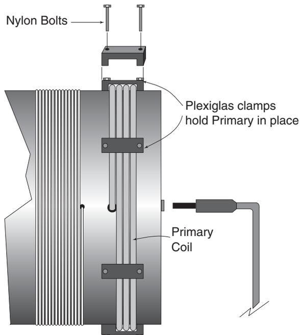
**Fig. 14 - Securing Primary Coil**
